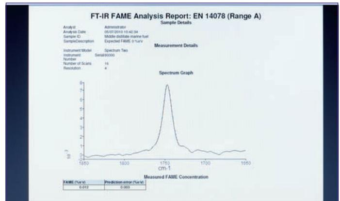
Regulated biodiesel measurement using application specific software.
