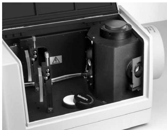
Fig. 1. The L6020322 Integrating Sphere (InGaAs) snap-in Module for the LAMBDA 1050.
