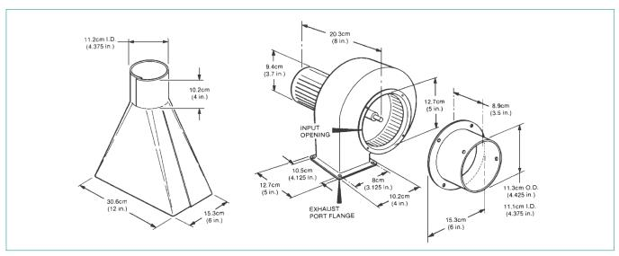
Figure 1. Blower and vent kit dimensions.
