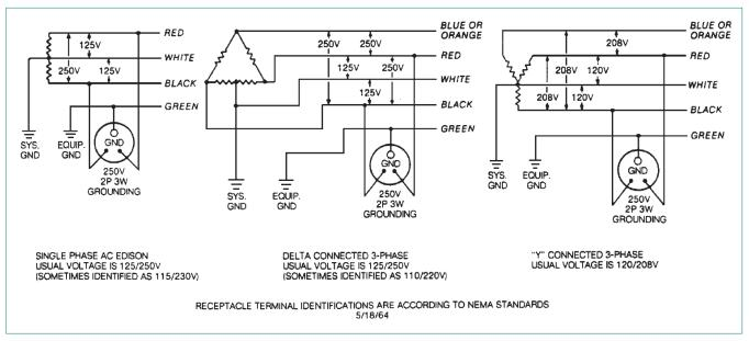
Figure 2. HGA power circuit connections.
