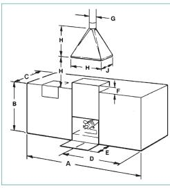
Figure 3. Spectrometer and accessories dimensions.
