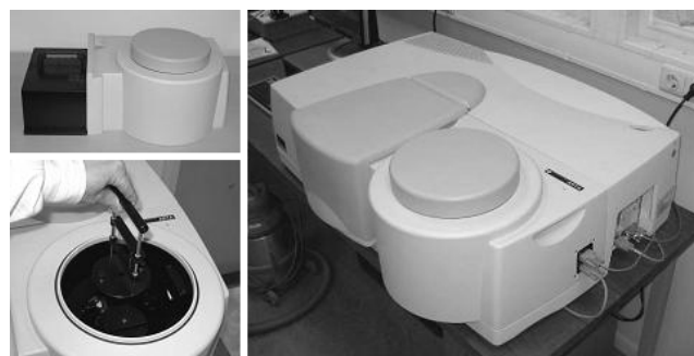
Fig. 2. The Automated Reflectance / Transmittance Analyser (ARTA) installed in the PerkinElmer Lambda 950 spectrophotometer.
