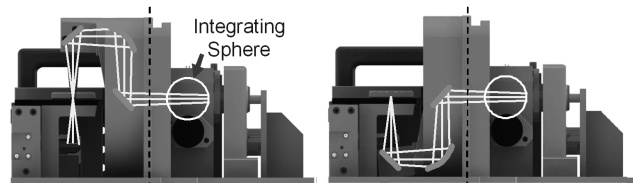
Fig. 19. Optical path of the beam between sample and detector sphere in transmittance (left) and reflectance (right).
