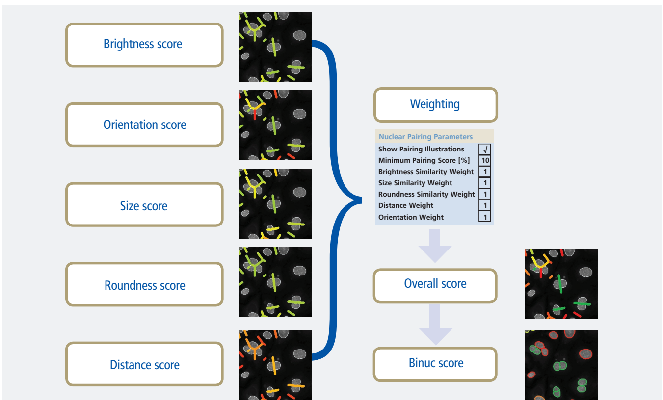
Figure 3. The Nuclear Pairing scoring system encompasses five measures (left), each of which contributes a factor in the assessment of all possible pairings of adjacent nuclei. These measures include assessment of the level of similarity between adjacent nuclei with respect to their size, brightness and roundness. The distance, which relates to the average diameter of the pair of nuclei being considered, and the orientation, which relates to the angle between the main axes of the two, is also assessed. Each measure is a contributing factor towards an overall score for each pairing. In the illustrations, the greener the line is, the higher the score, and the redder the line is, the lower the score. Yellow lines indicate score values where the pairing is just acceptable, as long as the average contribution from the other factors is not lower. The relative importance of the individual measures towards the overall score is determined by adjustable weights. For example, a weight of two would result in a factor being applied twice; whereas a zero weight would result in the measure being taken out of consideration. If the maximum score value is achieved, whereby the two nuclei touch each other and are equal in all examined properties, then this is considered to be a possible pairing of nuclei. The minimum score value that a pairing must reach in order to be accepted can be defined by the user as a fraction of this maximum. Yellow lines in the Overall score illustration indicate pairings with overall score values just above this limit. For each nucleus, the best possible and acceptable pairing is selected. If this is also the best pairing for the prospective partner then the pair is reconstructed into binuclear cells (Binuc score).
