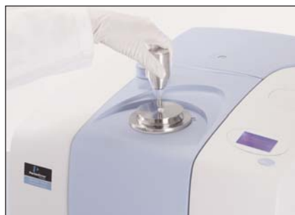
Figure 7. Applying pressure to a solid sample on the Universal diamond ATR top-plate.
