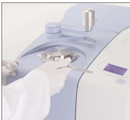
Figure 6. Placing a powder sample onto the Universal diamond ATR top-plate.
