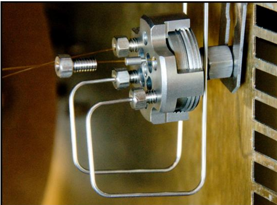
Figure 3. Assembly mounted on key-hole bracket in Clarus 600 GC oven and external connections being made.
