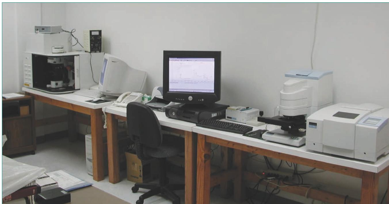
Figure 1. PerkinElmer Spectrum One FT-IR System and the AutoIMAGE microscope in the Microtrace laboratory.
