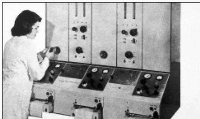
The **Model 188 Triplestage Gas Chromatograph**. The sample was introduced through the injection port of the leftmost unit and was then conducted by the carrier gas through three columns in series, each in a separate oven at different temperatures. Each had a thermal conductivity detector at the column outlet, making separate records of the particular fraction analyzed in that column.
