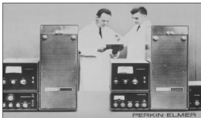
The **Model 810/820 Gas Chromatographs**. These represented advanced versions of the Model 800 Gas Chromatograph, originally introduced in 1962, offering, for the first time, dual-column baseline compensation in programmed-temperature operation, with differential flame-ionization detectors or with a dual thermal-conductivity detector. The Model 810 (on the left) is the FID and the Model 820 (on the right) is the TCD version.
