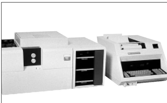
The microprocessor-controlled **Sigma 1 Gas Chromatograph** is shown with its data system on the right.
