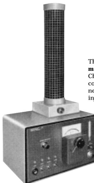
The **Model 222 Temperature Programming Accessory** for the Model 154 Gas Chromatographs. The resistance-heated column is behind the vertical "chimney." The injection port (for syringe injection) is just below the chimney.
