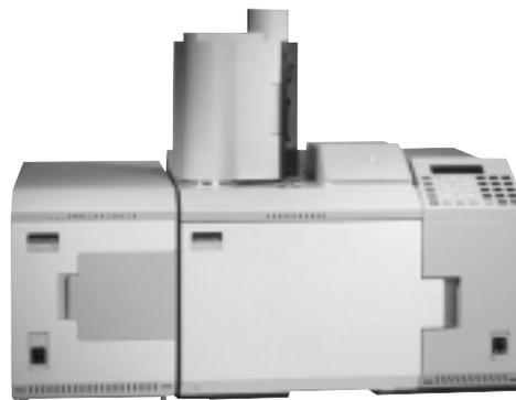
The **TurboMass Mass Spectrometer** is a quadrupole benchtop mass spectrometer with a standard mass range of 2-1200 daltons. It interfaces through the left side of the **AutoSystem XL Gas Chromatograph**, as shown in this photo.
