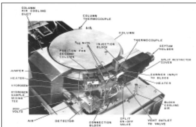
Configuration of the capillary column and heater of the **Model 226 Gas Chromatograph**. The heater is the disk at the bottom, while the capillary column is embedded in the disk above it.
