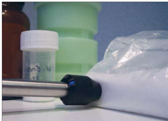
Figure 2. The nosepiece eliminates stray light and keeps the sample at the optimum focal distance from the probe.
