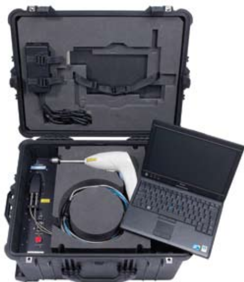
Figure 1. Raman IdentiCheck system allows positive identification of a wide range of sample types.
