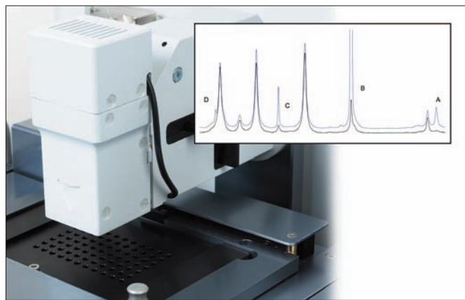
Figure 4. Showing polarization accessory and Raman spectra of cyclohexane arising from analysis Parallel (blue) and Perpendicular (black) to the excitation laser polarization. The large changes in peaks A-D signifies that these peaks arise from totally symmetric vibrations.
