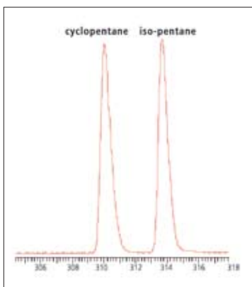
Figure 21. Critical separation 'B' – a good separation between these two compounds is critical.
