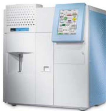
Figure 9. PerkinElmer TurboMatrix 100 TD system with online sampling accessory fitted on rear of instrument.
