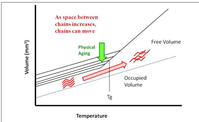
Figure 3. Free Volume in polymers is an basic principle for understanding behavior.
