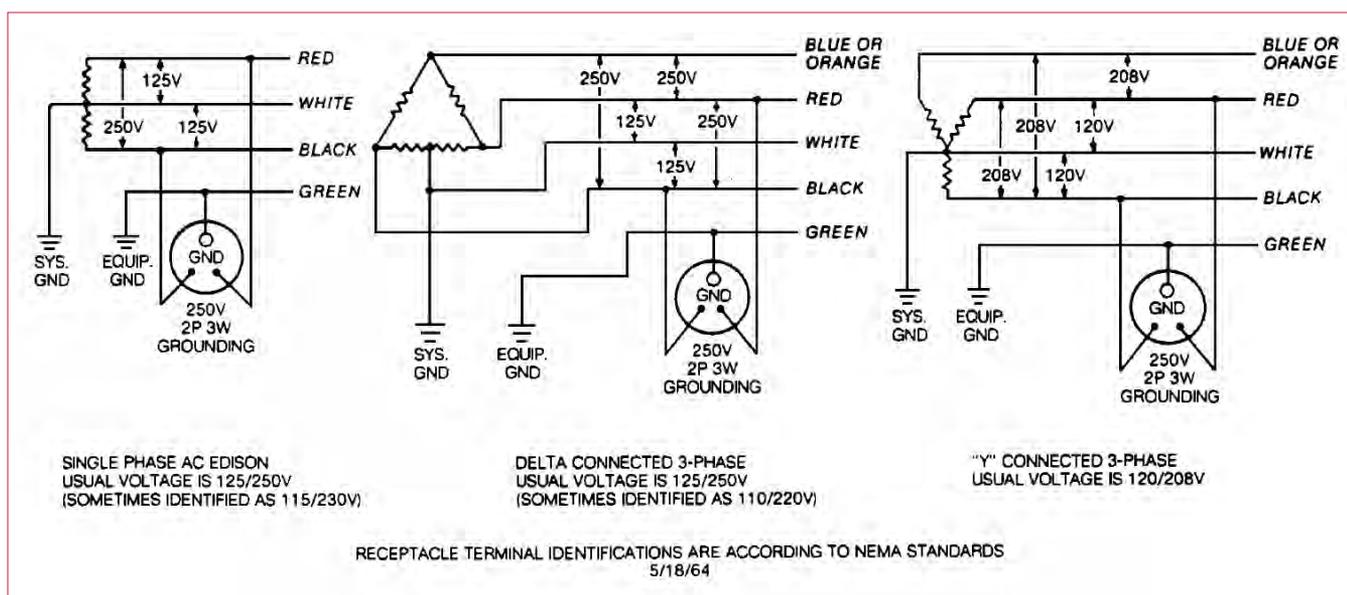
Figure 2. HGA power circuit connections.
