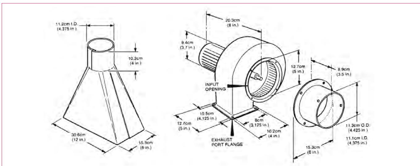
Figure 1. Blower and vent kit dimensions.
